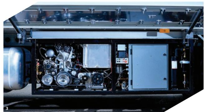
By using the liquid nitrogen engine as a secondary engine in trucks for cooling (instead of a second diesel engine), diesel consumption could be cut by up to 25%. The Dearman engine is also zero-emission and the company says it could one day be used in mass-market vehicles and for back-up cooling and power systems in buildings.
