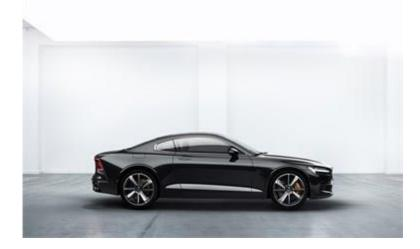
The Polestar 1 will form a halo for the future Polestar brand. The Polestar 1 is a two-door, 2+2 seat Grand Tourer Coupé with an 'Electric Performance Hybrid' drivetrain. An electric car supported by an internal combustion engine, it has a range of 150kms on pure electric power alone - the longest full electric range of any hybrid car on the market. Its output of 600hp and 1000Nm of torque places the car firmly in the performance car segment.
