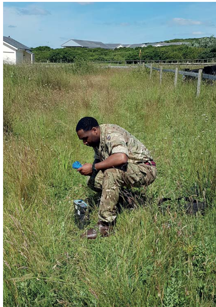
A student conducting soil resistivity in preparation of siting Field Power Station.
