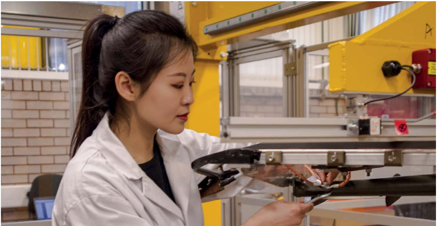
A researcher connects a pantograph test at the Birmingham Centre for Railway Research and Education.
