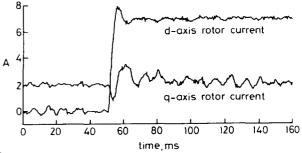
Fig.14 Experimental response to step change in d-axis rotor-current demand
