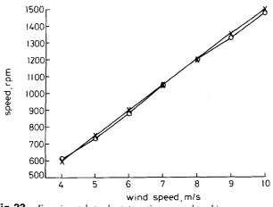
**Fig.23** Experimental steady-state optimum speed tracking \* optimum speed; O machine speed
