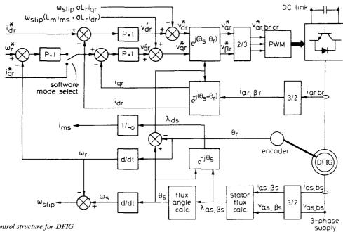
Fig. 10 Vector-control structure for DFIG
