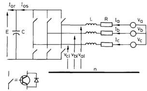
Fig.2 Supply-side converter arrangement
