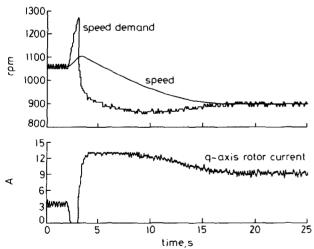
Fig.26 Experimental results results for driving into stall zone following a step increase in wind velocity
