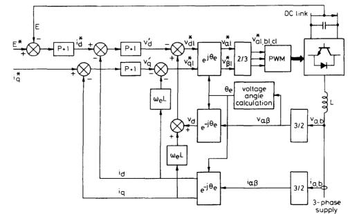
Fig. 3 Vector-control structure for supply-side converter
