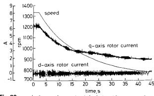
Fig.20 results for step decrease in wind velocity with current-mode control
