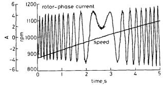
Fig. 17 Experimental results for operation through synchronous speed
