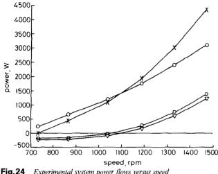
**Fig.24** Experimental system power flows versus speed  $\bigcirc$  Pstator;  $\square$  Protor;  $\triangledown$  Pfront - end;  $\divideontimes$  P - output
