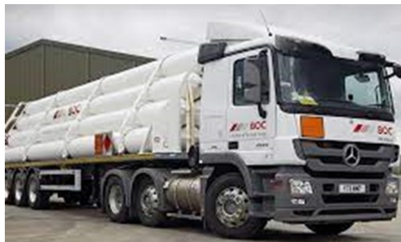
Figure 8 – Tube trailer for transporting hydrogen.
